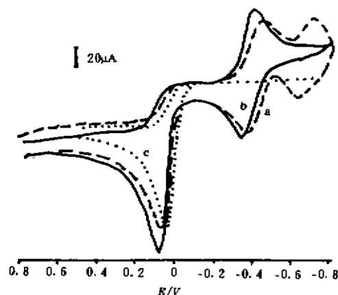
Fig. 1 Cyclic voltammograms of  $[\text{Mo}(\text{dte})_4][\text{Eu}(\text{dte})_4]$  (a),  $[\text{Mo}(\text{dte})_4][\text{Er}(\text{dte})_4]$  (b), and  $\text{Na}(\text{dte})$  (c) in DMF solution containing 0.1 mol/L  $\text{NaClO}_4$ . The scan rate is 50 mV/s and the scan range is from -0.8V to 0.8V.
