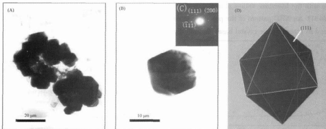
(A) at 450 °C; (B) with sizes around 10  $\mu\text{m}$ ; (C) The electron diffraction pattern;
