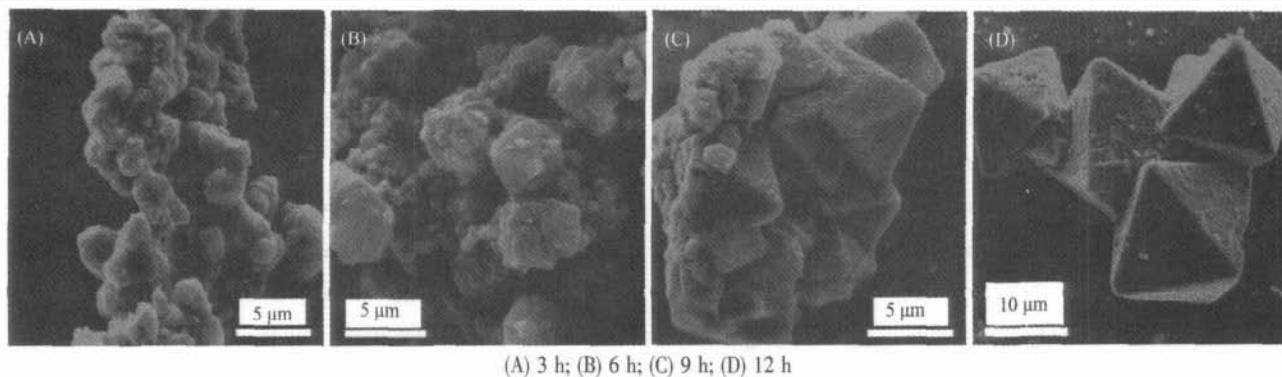
Fig.7 SEM images of particles of cobalt oxide grown at 450 °C during different time
