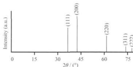
Fig.2 XRD standard pattern of cubic cobalt oxide
