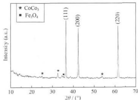
Fig.1 XRD pattern of a cobalt oxide powder sample prepared at  $450^\circ\text{C}$
