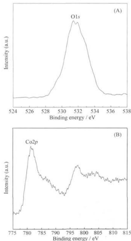
Fig.3 XPS Spectra of regular octahedron particles of cobalt oxide
