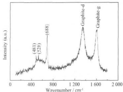
Fig.6 Raman spectrum of regular octahedron microcrystals of cobalt oxide, using an excitation wavelength of 514 nm
