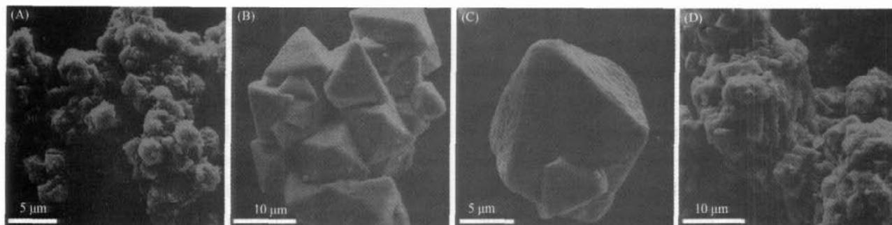
(A) grown at 400 °C; (B) regular octahedron grown at 450 °C;
