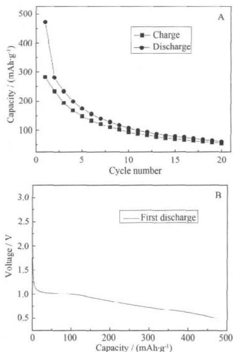
Fig.8 Effect of cycle number on the charge/discharge capacity of Li/CoO Teflon cell (A) and first discharge curve of Li/Co Teflon cell(B)
