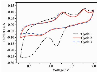
We firstly report nanostructured  $\text{Fe}_3\text{S}_4$  as a cathode material for rechargeable magnesium battery. Electrochemical tests show that the obtained  $\text{Fe}_3\text{S}_4$  can be reversibly cycled in rechargeable magnesium battery.
