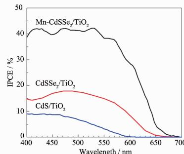
The Mn-CdSSe<sub>2</sub>/TiO<sub>2</sub> photoanode for quantum dots-sensitized solar cell (QDSC) was prepared by successive ionic layer adsorption and reaction method. In contrast to CdS/TiO<sub>2</sub> QDSC and CdSSe<sub>2</sub>/TiO<sub>2</sub> QDSC, the IPCE and energy conversion efficiency of Mn-CdSSe<sub>2</sub>/TiO<sub>2</sub> QDSC has increased evidently.
