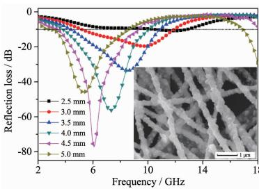
The electrospun  $(1-x)NZFO-(x)PZT$  magnetoelectric composite nanofibers with  $x=0.3$  and  $0.4$  exhibit better microwave absorption properties in the low- and high-frequency ranges, respectively, which may be attributed to the proper combination of magnetic loss of NZFO and dielectric loss of PZT, as well as the enhanced interfacial effects.
