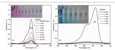
Four POM-based nanomaterials  $(PMo_{12}^{\ b},\ PW_{12}^{\ b},\ SiW_{12}^{\ b},\ GeW_{12}^{\ b})$  have been synthesized and present excellent adsorption properties of the organic dyes. The adsorption efficiency towards MB (100 mL of 20 mgL<sup>-1</sup>) could reach up to 96.3% in 5 min under dark condition, while it is up to 96.1% in 30 min towards RhB.
