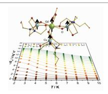
A family of {LnCu<sub>3</sub>} clusters were selected to study their magnetocaloric effect (MCE). The results suggest the importance of ferromagnetic interactions in designing of 3*d*-4*f* molecular coolers.
