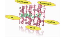
The crystallization process of AlPO<sub>4</sub>-12 was investigated using liquid NMR and electrospray ionization mass spectra (ESI-MS) and so on. The formation of 4-and 6-membered rings was confirmed by the ESI-MS data. These findings have important guiding significance for the directed synthesis of molecular sieves.
