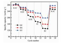
The  $\mathrm{Li}_{12}\mathrm{Mn}_{0.54}\mathrm{Ni}_{0.13}\mathrm{Co}_{0.13}\mathrm{O}_2$  materials with smaller second particle size showed a much superior rate capability to the sample with bigger particle size. The improvement in rate capability could be attributed to the smaller particle size, which gives a better contact between the active material and the electrolyte/conductive agent, at the same time a shorter diffusion path.
