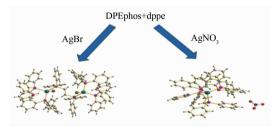
Complex 1 is comprised of AgBr, DPEphos and dppe (DPEphos =bis [2-(diphenylphosphino)phenyl]ether, dppe=bis(diphenylphosphino)ethane) in 2:2:1 molar ratio generating a binuclear complex. The dppe ligand bridges two Ag atoms through two P atoms. While, complex 2 is obtained by the reactions of AgNO<sub>3</sub>, DPEphos and dppe in 1:1:1 molar ratio generating a sample mono-nuclear complex.
