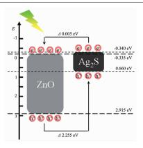
The presence of  $Ag_2S$  enhances the light absorption of the photocatalyst under the visible-light region and suppresses the growth of ZnO along the (001) crystal plane. When  $n_{Ag_2S}/n_{ZnO}$  was 1:10, the composite performs higher photocatalytic activity than P25 widely used at present.
