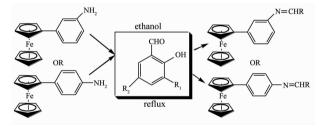
3-Ferrocenyl aniline and 4-ferrocenyl aniline were reacted with aromatic aldehyde in ethanol solution under reflux to produce 3-ferrocenyl phenyl imine and 4-ferrocenyl phenyl imine, respectively.
