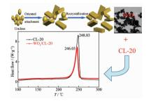
Based on the preparation of nanosized WO<sub>3</sub> cuboids, the effects of WO<sub>3</sub> cuboids on the thermal decomposition of CL-20 were investigated. WO<sub>3</sub> cuboids play an important role in reducing the peak temperature of the decomposition and the activation energy of CL-20.
