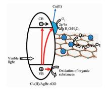
The highly efficient AgBr photocatalyst was developed with cooperation effect of Cu(II) cocatalyst and graphene as Cu(II) can catch electrons and graphene may provide a lot reduction active sites.
