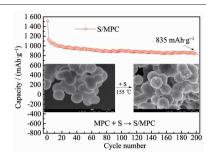
Sulfur/mesoporous carbon composites were achieved by melt infiltration of sulfur into mesoporous carbon which was prepared by template method. When the composites were applied as cathode material for lithium sulfur, the initial discharge specific capacity is as high as 1 519 mAh·g<sup>-1</sup>, and can remain 835 mAh·g<sup>-1</sup> even after 200 cycles.
