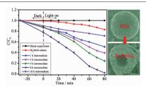
$Bi_2MoO_6$  photocatalyst with hollow structure was prepared by in-situ transformation method using BiOI as self-sacrificing template. The obtained  $Bi_2MoO_6$  hollow microspheres with specific surface area of 61 m<sup>2</sup>·g<sup>-1</sup> showed higher photocatalytic activity than that of  $Bi_2MoO_6$  sheets or the intermediates obtained at different reaction times.
