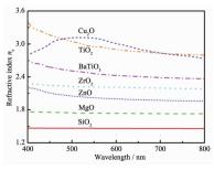
The SPR absorption position in visible region of the composite film is strongly dependent on  $n_{\rm s}$  rather than  $\varepsilon_{\rm ml}$  and  $\varepsilon_{\rm m2}$ . The simulated optical absorption spectra of the composite films dispersed by Ag, Au and Cu by Mie theory in this study are in good agreement with the reported experiment results, especially showing a close SPR peak positions to each other.
