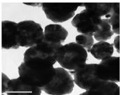
The nano nickel substituted cobalt ferrite hollow microspheres with uniform particle size and good dispersion were prepared by solvent thermal method. The average particle size is about 200 nm.
