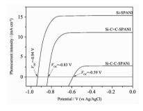
A strong photoelectric conversion rule was found in electrodes based on polyanilines with different substituted groups grafted on n-Si (111) crystalline surface, and a high photocurrent density of 15.4 mA  $\cdot$  cm $^{-2}$  and photoelectric transformation efficiency of 13.3% was obtained.
