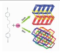
Complex 1 displays 2D→3D 3-fold interpenetrating framework with 4-connected sql topology; complex 2 shows a 3D 4-connected framework of 6<sup>6</sup> dia topology with 6-fold interpenetration. The magnetic properties of the two complexes indicate typical antiferromagnetic interactions.
