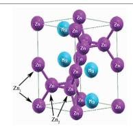
through interaction of two sp hybrid state, which are from Zn4s-4p hybridized orbit and Mg3s-3p hybridized orbit separately.  $MgZn_2$  phase shows paramagnetism, which stems mainly from the two unpaired electrons in the  $Zn_1$ -Mg bond.
