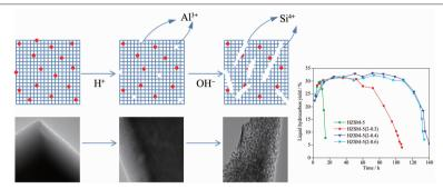
For ZSM-5 zeolite, the acid pre-treatment could facilitate formation of mesoporous structure in alkaline treatment process. With the increase of alkaline treatment intensity, the mesopore structure was increased and the strong acidity was decreased, which resulted in high catalytic activity and long lifetime for MTG reaction.
