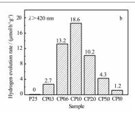
The effect of CuO loading on the reaction rate of photocatalytic hydrogen evolution was studied, by using UV-Visible light (a) and visible light (b) under irradiation of 300 W xenon lamp.
