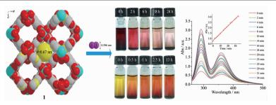
One metal-organic framework with regular porosity constructed from one acylamide tetracid ligand and copper ions exhibits an outstanding performance in reversible adsorption of iodine molecules. Two Different Co(II) Interpenetrating Networks Based on a Flexible Dicarboxylic Acid and Different Bis(imidazole) Ligands (English)
