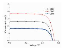
Basic optoelectronic characters and photovoltaic performances of three D- $\pi$ -A type organic dye sensitizers based on BODIPY derivatives featuring BODIPY as  $\pi$ -conjugate bridge, N-phenylcarbazole linked BODIPY unit with different active positions as electron donor and cyanoacrylic acid as electron acceptor were systematically investigated.
