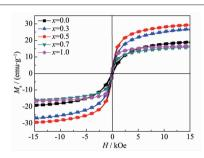
The monodisperse  $Ni_xZn_{1-x}Fe_2O_4$  nanoparticles show a typical ferrimagnetic behavior at room temperature. The maximum saturation magnetization with concentration of  $Ni^{2+}$  up to x=0.5 is determined to be 29.38 emu·g<sup>-1</sup>.
