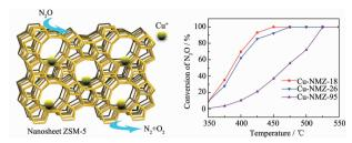
Cu-ZSM-5 nanosheets exhibit excellent activity and stability in  $N_2O$  decomposition. The catalytic activity in terms of TOF increases with the decreasing of the  $n_{\rm S}/n_{\rm Ah}$ , due to better reducibility of Cu<sup>+</sup> species and better desorption capability of adsorbed oxygen on catalysts with lower  $n_{\rm S}/n_{\rm Ah}$ .
