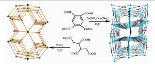
The 1,6-connected net of compound 1 and 2 is consisted of BETA<sup>4</sup> ligand with five-nuclear metal clusters. The BETA<sup>4</sup> ligand acts as a four-connected node, and each five-nuclear metal cluster acts as the other four-connected node. The BTCA<sup>4</sup> ligand as a eight-connected node in compound 3 are linked by  $Mn^{2+}$  ions to form 4,8-connected net.
