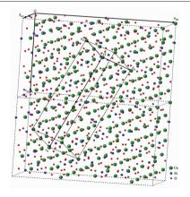
The superstructure of M3 modification in tricalcium silicate solid solution was described in detail. The orientation relations between M3 supercell and pseudohexagonal subcell was studied by computer simulation for the first time, and the conversion matrix between M3 supercell and pseudohexagonal subcell was established.
