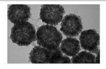
The Fe<sub>3</sub>O<sub>4</sub>@LDO particles possess well defined core-shell structure with Mg-Al Mixed Oxides as the shell and hollow  $Fe_3O_4$  particle as the core, and show high catalytic activity with yield of 62% in 2 h in the Knoevenagel condensation of benzaldehyde with ethyl acetoacetate.
