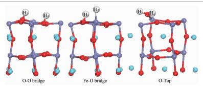
The study found that there are mainly three kinds of chemical adsorptions of H<sub>2</sub> molecules on the surface of LaFeO<sub>3</sub> (010): The first one is that H atoms is adsorbed to the O atom, forming -OH group; The second one is that one H atom is adsorbed to the Fe atoms, forming a metal bond; The last one is that two H atoms are adsorbed to the same O atom to form H<sub>2</sub>O molecules, and the H<sub>2</sub>O molecules can easily form oxygen vacancies.
