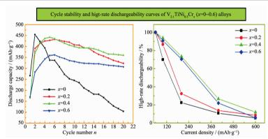
Cycle stability and high-rate dischargeability of  $V_{2.1} TiNi_{0.3} Cr_x$  (x=0~0.6) alloys were significantly improved by adding the Chromium.  $V_{2.1} TiNi_{0.3} Cr_{0.4}$  alloy with the high-rate discharge performance of 73.40% and the capacity retention rate of 81.91% showed the best electrochemical properties among the investigated alloys.
