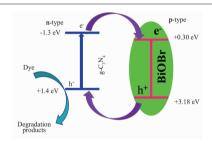
The heterostructure system with a firm interface of g-C $_3$ N $_4$ -BiOBr composite photocatalysts could efficiently separate the interfacial electron-hole pair and accordingly improve the visible-light photocatalytic activity.
