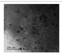
Active carbon doped by copper (0.7 mmol  $\cdot$  g<sup>-1</sup>) calcined at 300 °C under N<sub>2</sub> showed the best adsorption ability to mercaptan with low concentration because of the high surface area and well distributed Cu<sub>2</sub>O nanoparticles.
