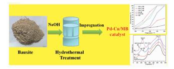
The bauxite pre-treated by NaOH solution was used as support. The physical-chemical properties and catalytic activities of the as-prepared Pd-Cu/MB catalysts for catalytic CO oxidation are modulated by the introduction of different amount of CuO.
