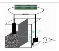
Photocatalysis supported by microbial electricity generation could greatly improve the reduction efficiency of nitrate. The result shows that this research could achieve synchronous implementation of biodegradation of sewage, electricity production and nitrate reduction with lower cost and better treatment effect.
