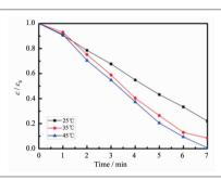
Using SiO<sub>2</sub> microspheres as hard template, Au@ZrO<sub>2</sub> hollow microspheres were prepared by deposition-precipitation method. p-Nitroaniline can be completely reduced to p-phenylenediamine in 7 minutes at 45 °C under the existence of the microspheres.
