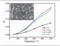
Bi doping is helpful for the sintering of  $\text{La}_{0.1}\text{Sr}_{0.9}\text{TiO}_3$  ceramics and make the grain fully developed, regularly shaped and combined closely. A remarkable ZT of 0.172 at 500 °C was obtained for the sample with x =0.075, which was increased by 130% compared with that of the sample without Bi.
