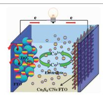
Co<sub>3</sub>S<sub>4</sub> supported by electrospun carbon nanofibers (Co<sub>3</sub>S<sub>4</sub>/ECs) composites with different weight of Co<sub>3</sub>S<sub>4</sub> on the surface of carbon nanofibers were synthesized by hydrothermal synthesis method and used as counter electrode for DSCs to study its photoelectric property.
