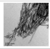
The carbon nanorods with ca. 20 nm in diameter and 200 ~800 nm in length were prepared through HNTs-templated nanocasting method, and mainly possessed two types of mesopores at 3.9 nm and 13.5 nm, respectively.
