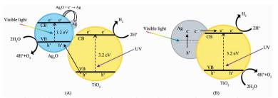
Prepared  $Ag_2O/TiO_2$  composites show enhanced photocatalytic  $H_2$  evolution rate, 15 times as high as that of P25, owing to the formation of heterojunction and presence of photo-induced Ag.
