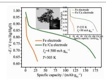
Fe/Cu nanocomposites endow excellent performance for nickel-iron batteries, significantly improve high-rate and lowtemperature performance.
