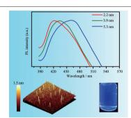
Monolayer MoS2 is the two-dimensional material which has the direct band gap, and has the excellent photoelectric properties. We have developed a heat-up route in oleylamine for the size-controlled synthesis of MoS<sub>2</sub> QDs and investigate the size effect of MoS2 on the fluorescence properties.
