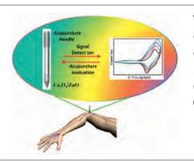
The Co<sub>3</sub>O<sub>4</sub>/ZnO acicular nanorod arrays (ANRAs) decorated acupuncture needle exhibits a high sensitivity of 2 264.27  $\mu$ A·L·mmol<sup>-1</sup>·cm<sup>-2</sup>, a fast response time (<4 s) and a detection limit as low as 0.311  $\mu$ mol·L<sup>-1</sup> (S/N=3).
