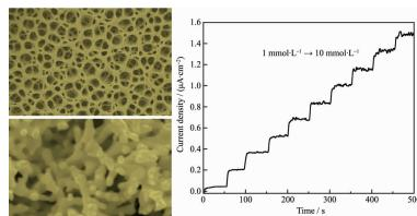
Herein, Au films with three-dimensional hierarchical pores were prepared by hydrogen bubble dynamic template method. The Au foam films show good electrocatalytic activities in enzyme-free detection of glucose.
