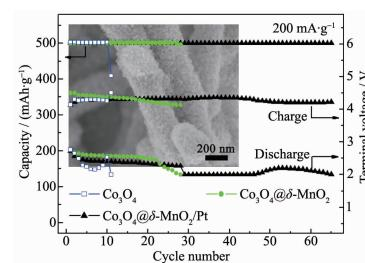
A binder-free array-type Co<sub>3</sub>O<sub>4</sub>@δ-MnO<sub>2</sub>/Pt catalytic cathode exhibits high catalytic effect for oxygen reduction/evolution reactions, enabling conformal growth of thin-layered Li<sub>2</sub>O<sub>2</sub> and long cycle life of the Li-O<sub>2</sub> cell.
