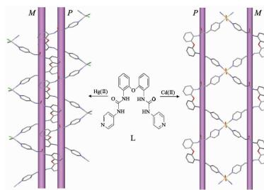
Two coordination polymers  $\{[\text{Hg}(\text{L})\text{Cl}_2] \cdot 2\text{DMF}\}_n$  (**1**) and  $\{[\text{Cd}(\text{L})_2(\text{H}_2\text{O})_2](\text{ClO}_4)_2 \cdot 4\text{DMF} \cdot 2\text{H}_2\text{O} \cdot 2\text{CH}_3\text{OH}\}_n$  (**2**) were synthesized and characterized. Their structures were measured via single crystal X-ray diffraction and their thermal stabilities and vapor adsorptions for MeOH were further investigated.
