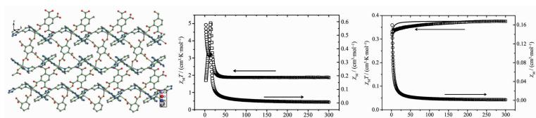
The present work reports synthesis and characterization of two new isomorphic coordination polymers,  $[\text{M}(\text{btec})_{0.5}(\text{H}_2\text{L})]_n$  ( $\text{M}=\text{Co(II)}$  (**1**),  $\text{Cu(II)}$  (**2**)). Compounds **1** and **2** are 2D structure. In addition, magnetic studies indicate that **1** show weak ferromagnetic between metal ions and there is typical paramagnetic behavior in **2**.
