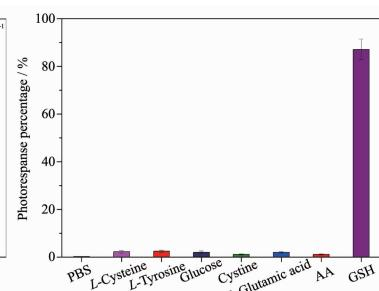
The BiVO<sub>4</sub> thin films (~120 nm in thickness) exhibits an excellent visible-light PEC performance for both the water splitting and detection of the glutathione (GSH) with ultralow contents.
