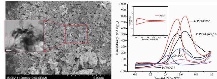
2D structure of WS<sub>2</sub> and anchoring effect of NaCl were used to fabricate the porous WC/C flakes. The Pt/WC/C shows good electrocatalytic activity, stability and excellent resistance to CO poisoning in MOR.
