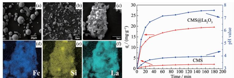
The obtained CMS@La<sub>2</sub>O<sub>3</sub> exhibit a high P adsorption capacity of 19.50 mg·g<sup>-1</sup> and could be easily magnetically separated from aqueous solution.
