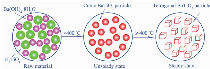
Submicron tetragonal BaTiO<sub>3</sub> with well homogeneity and dispersion has been prepared by solid state reaction at low temperature of 400 °C, which can effectively reduce energy consumption and waste liquid production.
