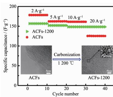
After the activated carbon fibers (ACFs) were modified by carbonization, the degree of crystallinity of ACFs were enhanced and the conductivity was effectively improved. The ACFs carbonized at 1200 °C (ACFs-1200) electrodes show a high capacity retention at high current densities.
