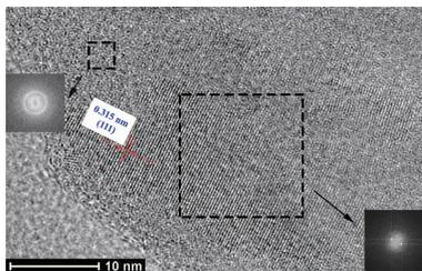
Both crystalline regions and amorphous regions are exhibited as labeled in the TEM image of the Si powders milled for 1 h, which demonstrates that the elongated ball milling time makes crystalline silicon to transform into partial amorphous phase.
