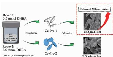
The rod-like and sheet-like CeO<sub>2</sub> were successfully synthesized with different amount of 2,4-dihydroxybenzoic acid (DHBA) as auxiliary. The rod-like CeO<sub>2</sub> manifested the better catalytic activity in NH<sub>3</sub>-SCR.
