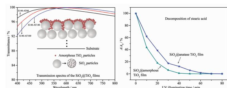
The SiO<sub>2</sub>&amorphous-TiO<sub>2</sub> anti-reflective films show an exceptional photocatalytic activity even higher than the counterparts with anatase phase.
