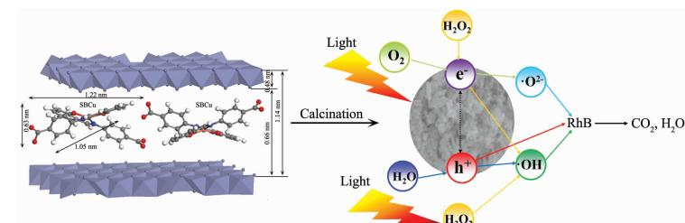
Zn-Cr-Cu composite metal oxides derived from hybrid Layered double hydroxides as a novel photocatalytic material exhibits a better photocatalytic activity for RhB degradation under the synergistic effect of H<sub>2</sub>O<sub>2</sub>.
