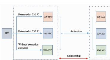
Different activated carbons were prepared by diverse hyper-coal extracted in different temperatures. The relationship is discussed between the functional groups in hyper-coal and the pore structure as well as electrochemical performance of the activated carbon.
