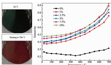
With testing temperature increasing from room temperature to 700 °C, the ZnO powders doped by Co<sup>2+</sup> ions change reversibly from green to tawny. Meanwhile, the emissivity increases gradually, and the maximum variation reaches 0.447.
