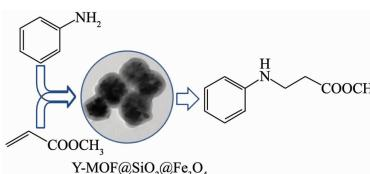
The catalyst performance of a core-shell magnetic Y-MOF@SiO<sub>2</sub>@Fe<sub>3</sub>O<sub>4</sub> catalyst for Aza-Michael addition reaction with aniline and methyl acrylate was evaluated, and exhibited good reusability and good superparamagnetism.
