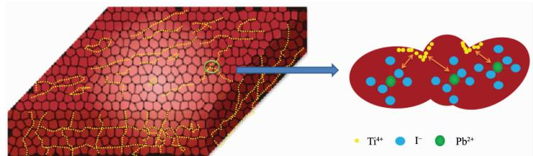
Ti<sup>4+</sup> formed at the grain boundary to passivate the defects of polycrystalline perovskite film. The performance of perovskite solar cells is effectively improved.
