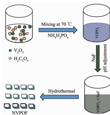
A simple hydrothermal preparation method was developed, regulating the morphology and size of the NVPOF by adjusting the key parameters including the pH value and hydrothermal temperature. The optimized NVPOF material exhibits the highest particle-size uniformity and thereby the best electrochemical properties.
