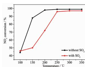
Mo-Ce/GE catalyst demonstrated excellent catalytic activity in NH<sub>3</sub>-SCR, because the addition of Mo can increase  $n_{\text{Ce}^{3+}}/(n_{\text{Ce}^{3+}} + n_{\text{Ce}^{4+}})$ , the oxygen content and the acid sites. In addition, the activity declined significantly (<250 °C) and remained unchanged (>250 °C) due to the formation of SO<sub>4</sub><sup>2-</sup> enhancing the acidity in the presence of SO<sub>2</sub>.
