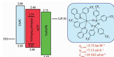
A novel iridium complex  $\text{Ir}(\text{tfmipi})_2(\text{tfmtpip})$  has been successfully applied in OLEDs (ITO/TAPC(40 nm)/ $\text{Ir}(\text{tfmipi})_2(\text{tfmtpip})(4\%)$ :mCP(20 nm)/TmPyPB(40 nm)/LiF(1 nm)/Al(100 nm)). The EL performances ( $\eta_{c,\max}=7.13 \text{ cd} \cdot \text{A}^{-1}$ ,  $\eta_{p,\max}=5.73 \text{ lm} \cdot \text{W}^{-1}$ ) are obtained.
