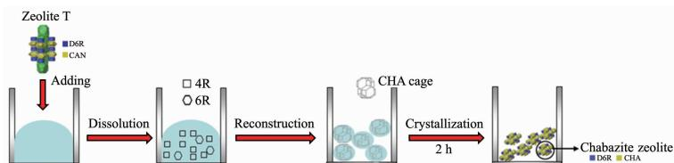
Low-silica chabazite zeolites were fast synthesized by adding zeolite T within only 8 h. Pure-phase chabazite zeolites showed the typical walnut-like morphology with particle size of ~1.5  $\mu\text{m}$ . Crystallization mechanism of chabazite zeolites induced by heterogenous seeds was investigated.
