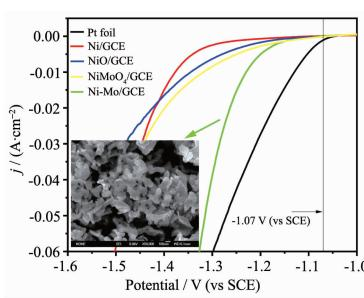
The nanoporous Ni-Mo alloy prepared by de-alloying has the highest hydrogen evolution activity. Its exchange current density is  $0.25 \text{ mA} \cdot \text{cm}^{-2}$ , and its hydrogen evolution over-potential increases only 39 mV after 10 000 s constant current density electrolysis, showing excellent hydrogen evolution stability.
