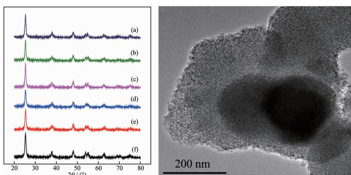
Mesoporous titanium dioxide (m-TiO<sub>2</sub>) and rGO/m-TiO<sub>2</sub> samples were synthesized. When  $w_{\text{GO}}/w_{\text{TiO}_2}$  was 0.01, the hydrogen production rate of rGO/m-TiO<sub>2</sub> was 241 mmol  $\cdot \text{g}^{-1} \cdot \text{h}^{-1}$  under UV light irradiation, and 9 mmol  $\cdot \text{g}^{-1} \cdot \text{h}^{-1}$  under visible light irradiation.
