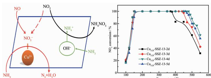
Cu-SSZ-13 catalysts with different crystallization time have been synthesized via one pot *in-situ* synthesis. Proper crystallization time leads to the proper copper species content and great distribution of active copper species, which contributes to the excellent NH<sub>3</sub>-SCR activity.
