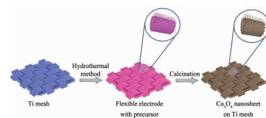
The layered  $\text{Co}_3\text{O}_4$  nanosheet arrays on Ti mesh with porous surface were adopted to optimize the transfer resistance and improve electrochemical performance of the flexible electrode.
