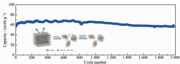
A novel easily-scalable “top-down” method was used to prepare graphite cathode materials with characteristics of few layers, small size and defect-free, which further increases the embedding sites of ions and breaks the inherent capacity limitation of graphite, so as to improve the electrochemical performance of aluminum ion batteries.
