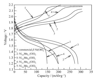
Manganese-doped Ni<sub>1-x</sub>Mn<sub>x</sub>(OH)<sub>2</sub> was prepared by buffer solution method. The constant current charge-discharge tests show that the material of Ni<sub>0.8</sub>Mn<sub>0.2</sub>(OH)<sub>2</sub> had excellent cycle performance and exhibited a high specific discharge capacity of 288.8 mAh·g<sup>-1</sup> at 800 mA·g<sup>-1</sup> when the specific discharge capacity of commercial β-Ni(OH)<sub>2</sub> was 198.7 mAh·g<sup>-1</sup>.
