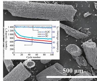
A highly-ordered carbon tube (OCT) was prepared via a facile method and possessed high specific area and pore volume. The as-prepared material exhibited superior electrochemical performances for lithium sulfur battery.
