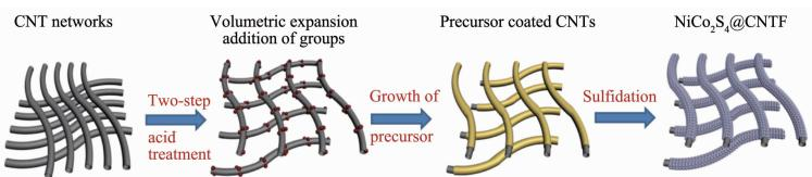
A new top-down route was reported to the synthesis of  $\text{NiCo}_2\text{S}_4@\text{carbon}$  nanotubeconstructed flexible composite film electrodes with good structure integrity even after repeated large deformations, a high capacitance of  $270.3 \text{ mF} \cdot \text{cm}^{-2}$  at  $0.5 \text{ mA} \cdot \text{cm}^{-2}$  and outstanding cycle life (93% of initial capacitance after 10 000 cycles at  $2.5 \text{ mA} \cdot \text{cm}^{-2}$ ).
