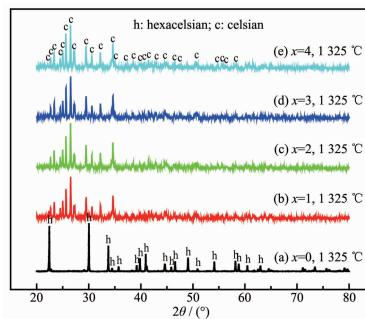
BAS-x% (*w/w*) LNBS (*x*=0, 1, 2, 3, 4) ceramics were prepared by solid state route. The phases structure were examined by X-ray diffraction, indicating that Li<sup>+</sup> substituting for Al<sup>3+</sup> or Li<sup>+</sup> entering into the single four-membered-ring(S4R) could promote the hexacelsian-to-celsian transformation by doping LNBS sintering aids.
