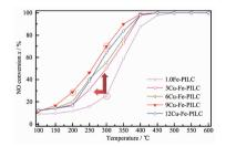
The modification of copper significantly improved the SCR-HC activity of the iron pillared montmorillonite catalyst at medium and low temperature.
