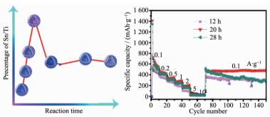
The percentage ratio of Sn to Ti can be adjusted by the reaction time during a solvothermal synthesis of SnO<sub>2</sub>/TiO<sub>2</sub> hollow microspheres, and SnO<sub>2</sub>/TiO<sub>2</sub> microspheres exhibit good electrochemical properties in lithium ion batteries.
