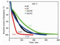
As 97% of the theoretical capacity released within 92 min, the hydrogen release rate of S5 samples increased by 178%. According to the isothermal hydrogen release curve of the second cycle, the secondary hydrogen release rate of S5 samples was still 40% higher than that of the original sample(S0).
