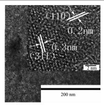
Co<sub>9</sub>S<sub>8</sub>/ZnS/C The flake composites prepared by solvothermal method, has high electrocatalytic oxygen production performance, which can be attributed to a small amount of inert ZnS components and pore structure of the composite.
