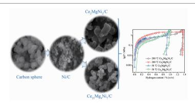
Solvent-thermal synthesis of Ce-Mg-Ni/C nano-composite material comprising  $Ce_2MgNi_2$  or  $Ce_{23}Mg_4Ni_7$  ternary alloy phase was reported. Hydrogen adsorption capacity of these composites reached 1.54% and 1.05%(w/w) at 50 °C, respectively.
