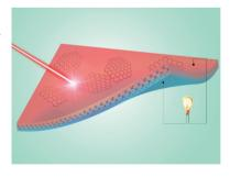
A novel photo-thermoelectric nanogenerator (PTENG) was designed utilizing a flexible pyroelectric polymer film with dispersed molybdenum disulfide. The incident near-infrared light energy is harvested by the transition-metal dichalcogenide as thin-layered nanosheets and converted into thermal energy. The pyroelectric polymer subsequently transduces the thermal energy into electric energy.
