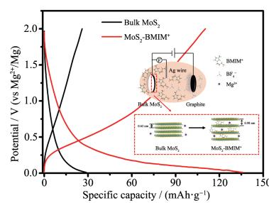
The micro-sized MoS<sub>2</sub> intercalated compound was prepared by a simple electrochemical method and used as cathode material of magnesium ion batteries. The MoS<sub>2</sub>-BMIM<sup>+</sup> showed a significantly improved specific capacity (101.93 mAh·g<sup>-1</sup> at 20 mA·g<sup>-1</sup>, about 4 times as much as bulk MoS<sub>2</sub>).
