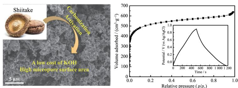
Shiitake - derived nitrogen - rich microporous carbons presented a high micropore surface area of  $1\text{ }594\text{ m}^2\cdot\text{g}^{-1}$ , a high capacitance of  $325\text{ F}\cdot\text{g}^{-1}$  at  $0.5\text{ A}\cdot\text{g}^{-1}$ , good rate capability, and robust stability.
