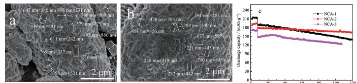
With the addition of PVP and PEG, the growth of primary grains is improved, resulting in the excellent electrochemical performance of NCA which displayed a high discharge capacity of 210.8 and 188.9  $\text{mAh} \cdot \text{g}^{-1}$ , and showed good capacity retention of 78.8% and 93.2% after 100 cycles.
