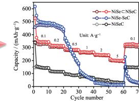
NiSe nanocrystallines confined within a N,Se-codoped carbon scaffold are readily *in-situ* fabricated via a two step direct solid state reaction, which demonstrate exceptional electrochemical performances as anode materials for sodium-ion batteries.
