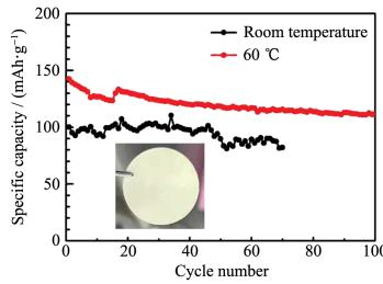
A solid composite electrolyte possesses a high ionic conductivity of  $1.14 \times 10^{-4}$  S·cm<sup>-1</sup>. The LiFePO<sub>4</sub>/Li cell with solid electrolyte exhibits a discharge capacity of  $100.1\text{ mAh}\cdot\text{g}^{-1}$  and a high capacity retention rate of 82% after 70 cycles at 0.1C.
