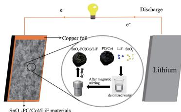
The porous carbon (PC(Co)) scaffold was used to host SnO<sub>2</sub> as a collector. Among them, the cobalt oxide in the PC(Co) material can enhance the electrochemical kinetics, but consume a certain amount of lithium ions. In order to ensure the superiority of batteries performance, LiF was added as a supplement to the lithium source.
