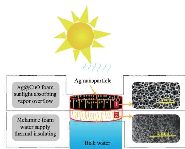
Multi - scale Ag/CuO composites were prepared by *in - situ* chemical reaction, heat treatment and evaporative deposition technology and applied to interfacial photothermal desalination successfully. The effects of light trap structure design and novel metal doping on the properties of metal - based composite photothermal materials were explored.
