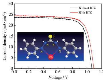
Dithizone (DTZ) post-treatment can improve the performances of organic-inorganic hybrid perovskite solar cells. DTZ can not only improve the morphology of the perovskite film by inducing its secondary crystallization, but also can passivate the Pb defects by forming the Lewis acid-base adducts through covalent bond between nitrogen atoms and Pb<sup>2+</sup>.
