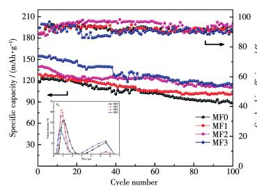
Mn-doped LiFePO<sub>4</sub> had smaller particle size and better electrochemical performance compared with pure phase LiFePO<sub>4</sub>.
