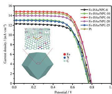
N-doped porous carbon (NPC) loaded with isolated single Fe atom (Fe-ISAs/NPC) was prepared through molecular cage-encapsulated-precursor pyrolysis. Meanwhile, film thickness of counter electrode effect on the performance of DSSCs was studied by electrochemical measurement.
