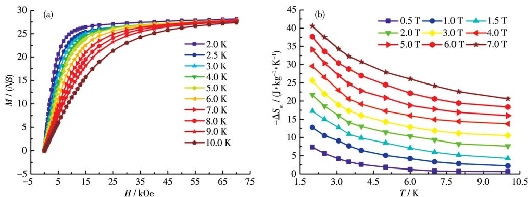
Fig.6 (a)  $M$  vs  $H$  plots for **1** at  $T=2.0-10.0$  K and  $H=0-70$  kOe; (b) Plots of  $-\Delta S_m$  vs  $T$  for cluster **1**
