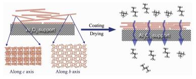
Open-pore MFI nanosheets were deposited on  $\mathrm{Al}_2\mathrm{O}_3$  support to make an isotherm selective MFI nanosheet membrane.
