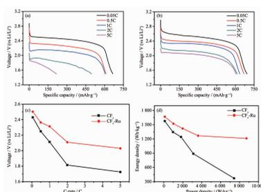
The ruthenium-modified fluorocarbons as anode material of lithium primary battery showed excellent rate capability and energy density, which is attributed to the removal of inert groups and the increase of specific surface area during the introduction of ruthenium.
