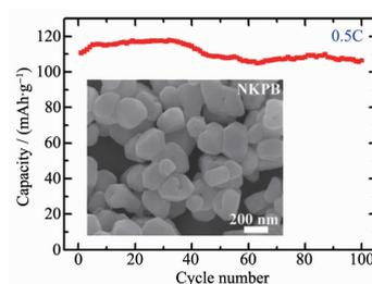
A Na-doped K-based Prussian blue material  $K_{1.9}Na_{0.1}Mn[Fe(CN)_6] \cdot 0.4H_2O$  prepared by an ion-exchange method showed a high capacity of  $136.3 \text{ mAh} \cdot \text{g}^{-1}$  at 0.1C, good rate capability of  $68.4 \text{ mAh} \cdot \text{g}^{-1}$  at 10C and good cycling stability with 96.1% capacity retained after 100 cycle at 0.5C.
