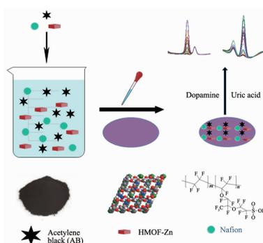
The GCE electrode modified by a kind of chiral MOF blended with acetylene black that fixed by Nafion had a high electrical signal response to dopamine and uric acid. Dopamine and uric acid can be simultaneously detected on the modified GCE electrode and totally independent of each other.
