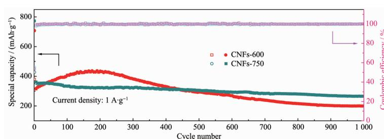
The type and content of nitrogen in CNFs prepared at different carbonization temperature can improve the storage performance of Li<sup>+</sup> in LIBs, and then improve the capacity of electrode.
