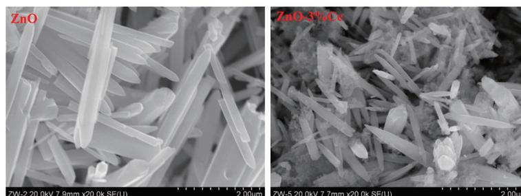
Moderate doping of Ce<sup>3+</sup> can change the morphology of nano-ZnO and greatly improve the photocatalytic degradation activity of organic dyes
