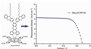
The antenna molecule S3 effectively enhances the spectral responsiveness of the DSSC, making the conversion efficiency increase by 1.2 times.
