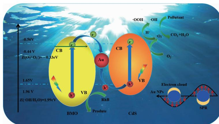
Z-scheme CdS/Au/Bi<sub>2</sub>MoO<sub>6</sub> heterostructure have been successfully fabricated by co-modification with CdS and Au on the surface of Bi<sub>2</sub>MoO<sub>6</sub>, thus significantly improving photocatalytic activity of Bi<sub>2</sub>MoO<sub>6</sub>.
