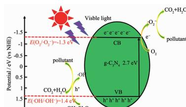
$\alpha$ -HNO<sub>3</sub>-g-C<sub>3</sub>N<sub>4</sub> which had high catalytic activity and stability was synthesized from the activation of melamine by HNO<sub>3</sub>. A multilayered buildup structure was formed, which increased specific surface area and pores volume of sample. Consequently, the carrier transport capacity was significantly enhanced, and band gap dropped to 2.7 eV.
