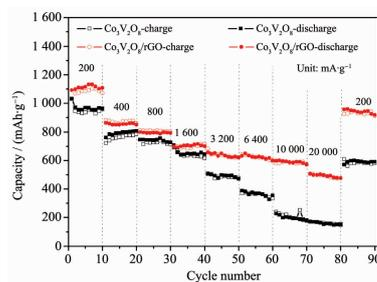
The  $\text{Co}_3\text{V}_2\text{O}_8/\text{rGO}$  composite has been successfully prepared by through a facile hydrothermal combined thermal treatment method. The excellent electrochemical performance is attributed to the synergistic effect from reduced graphene oxide and  $\text{Co}_3\text{V}_2\text{O}_8$ , and the composite structure can improve the electrode conductivity and efficient buffering the volume change.
