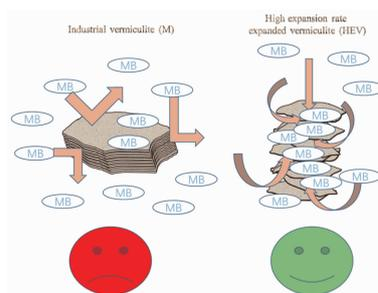
To improve vermiculite application efficiency and broaden its application field, we prepared HEV and tested its adsorption effect on MB. The results showed that the MB adsorption capacity of HEV was higher than that of some natural clay minerals and commercial grade activated carbon.
