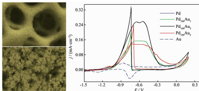
Three-dimensional (3D) porous Au-doped PdAu alloy foam films were obtained by using a hydrogen bubble dynamic template electrodeposition method. The Au-doped PdAu alloy foam films showed high electrocatalytic activity toward the electrooxidation of ethanol in alkaline media.
