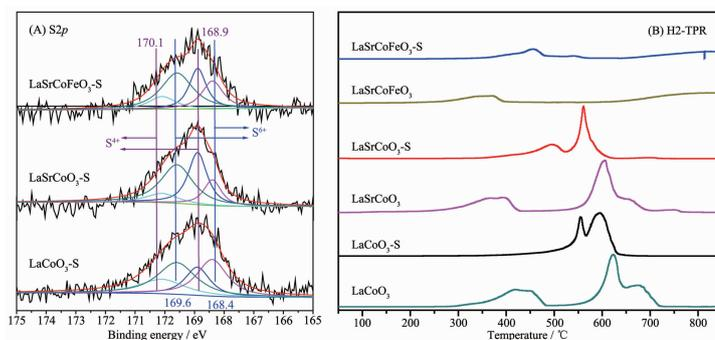
The catalysts exhibited excellent catalytic oxidation soot activity and sulfur resistance. Moreover, the poisoning of  $\text{SO}_2$  was mainly attributed to the sulfation ( $\text{SO}_3^{2-}$ ,  $\text{SO}_4^{2-}$ ) of  $\text{Co}^{2+}/\text{Co}^{3+}$  and surface adsorbed oxygen, leading to deactivating the active site ( $\text{O}_2^-$  or  $\text{O}^-$  and  $\text{Fe}^{4+}$ ) of catalyst.
