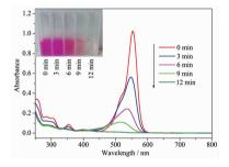
The heterojunction photocatalyst of g-C<sub>3</sub>N<sub>4</sub>@BiOCl with hollow flower-like structure was fabricated and exhibited much higher photocatalytic activity than g-C<sub>3</sub>N<sub>4</sub> and BiOCl under visible-light irradiation ( $\lambda \ge 420$  nm). The degradation efficiency of 50 mg·L<sup>-1</sup> rhodamine B can be reached to 99% within 12 min.
