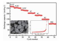
The porous micro-nano Li-rich  $0.6 \text{Li}_2 \text{MnO}_3 \cdot 0.4 \text{LiNi}_{0.5} \text{Mn}_{0.5} \text{O}_2$  cathode has well-ordered layered  $\alpha$ -NaFeO<sub>2</sub> structure and high BET specific surface area (13 m<sup>2</sup> · g <sup>-1</sup>), which endows the significantly improved high performance (10C, 107 mAh ·g -1) and cycling stability (94% of capacity retention at 0.5C after 100 cycles).
