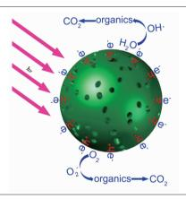
The porous ZnO/BiOI microspheres showed high photodegradation activities whether in RhB aqueous solution or in CH<sub>3</sub>CHO gaseous phase.
