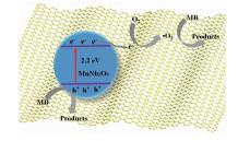
The as-prepared RGO-MnNb<sub>2</sub>O<sub>6</sub> composites could significantly enhance photocatalytic activity for the degradation of methylene blue under visible light irradiation. Within 60 min, 78.2% of the methylene blue was removed by the optimum sample (3% RGO-MnNb<sub>2</sub>O<sub>6</sub>), which was about 2 times higher than that of the individual  $MnNb_2O_6$ .
