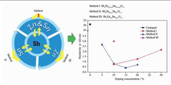
By the three substitution methods (I, II and III), the Sb ions successfully entered into the lattice positons of the target ions as designed, resulting in the variation of the conductivity of the Sb-doped ZTO films.
