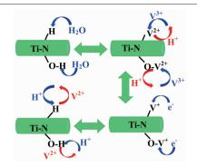
TiN NTs electrode provides large electrochemical surface area and more active center to improve the absorption of V(III), therefore the TiN NTs electrode exhibited excellent electrochemical activity towards V(III)/V(III) redox couple.
