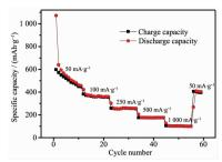
3DOM Fe<sub>2</sub>SiO<sub>4</sub>/SiO<sub>2</sub>@C nano-glass-ceramic exhibits a highly reversible discharge capacity up to 450 mAh·g<sup>-1</sup> at a current density of 50 mA·g<sup>-1</sup>, and 260 mAh·g<sup>-1</sup> at 250 mA·g<sup>-1</sup> in the voltage range of 0.05~3.0 V, while 3DOM amorphous SiO<sub>2</sub>@C composite with same porous structure only delivers 15 mAh·g<sup>-1</sup> at 50 mA·g<sup>-1</sup>.
