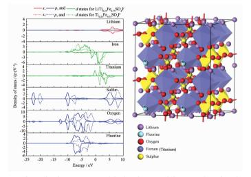
Ti doping results in the disappearance of the band gap, and then significantly enhances the electric conductivity and structural stability of LiFeSO $_4$ F cathode materials.
