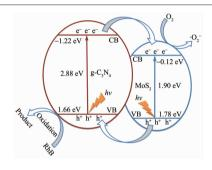
The MoS<sub>2</sub>/g-C<sub>3</sub>N<sub>4</sub> composites with significantly enhanced visible light photocatalytic performances were fabricated through combining the exfoliated commercial MoS<sub>2</sub> with g-C<sub>3</sub>N<sub>4</sub>.
