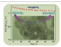
Nano-sized  $CeO_2$  particles embedded in the amorphous  $ZrO_2$  matrix for recycling of  $Cl_2$  from HCl oxidation, which are thus prevented from sintering during the reaction.
