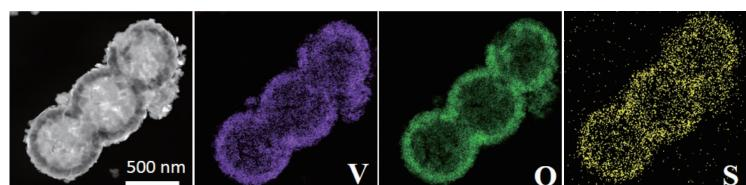
$\text{V}_2\text{O}_5$  hollow spheres were synthesized by hydrothermal synthesis and annealing as high efficient sulfur host for high performance lithium-sulfur batteries which can storage more sulfur and effectively restrict the shuttle effect of polysulfides.
