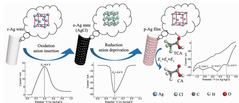
Voltammetric etching using chloride ion was employed to fabricate a highly activated polyporous silver film for electrochemical detection of trichloroacetic acid.
