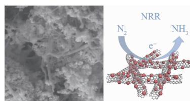
Low-cost catalyst carbon nanotube-based double transition metal nitrides  $\text{Co}_3\text{W}_3\text{N}/\text{CNTs}$  composite with small particle size was synthesized, which shows excellent ammonia production rate, Faraday efficiency and long-time electrochemical stability during nitrogen reduction reaction.
