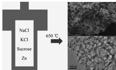
NaCl/KCl molten salts zinc-thermal method was used to prepare three-dimensional (3D) porous carbon materials with sucrose as precursor, which exhibits excellent rate performance and long cycle life for PIBs.
