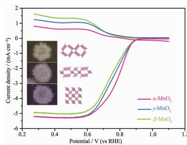
The effect of urchin-like  $\text{MnO}_2$  microspheres with three crystalline phases on oxygen reduction reaction was studied, and the activity followed a sequence:  $\alpha\text{-MnO}_2 > \gamma\text{-MnO}_2 > \beta\text{-MnO}_2$ . The difference of the activities was mainly related to the amount of  $\text{Mn}^{3+}$ , surface oxygen vacancies and conductivity.
