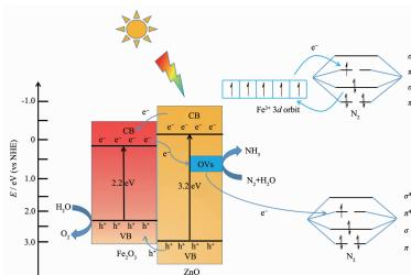
$\text{Fe}_2\text{O}_3/\text{ZnO}$  catalysts exhibited photocatalytic nitrogen fixation efficiency due to the enhancement of visible light absorption, higher concentration of surface oxygen vacancies and  $\text{Fe}^{3+}$  active sites.
