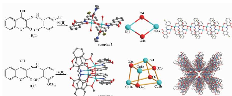
Two Schiff base binuclear Ni(II) and cubane-like Cu<sub>4</sub>(μ<sub>3</sub>-O)<sub>4</sub> core tetranuclear Cu(II) complexes formed the 1D supramolecular chain and the 3D network supramolecular structure, respectively, by different intermolecular interactions.
