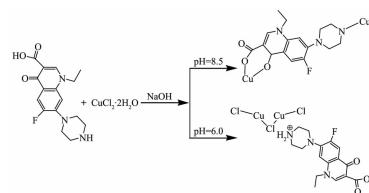
Under alkalinity and acidity conditions, two different copper complexes  $[\text{Cu}_2(\text{HNOR})_2\text{Cl}]_n$  (**1**) and  $[\text{Cu}_2\text{Cl}_3]\cdot\text{H}_3\text{NOR}\cdot\text{H}_2\text{O}$  (**2**) were obtained, respectively.
