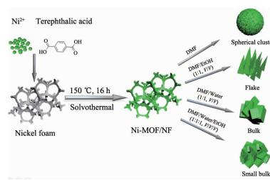
Direct growth of Ni-MOF material on the surface of nickel foam was achieved via a simple one-step solvothermal method. Solvents have remarkable effect on the morphology and electrochemical performance of the Ni-MOF/NF because of their different pH values and solubilities of terephthalic acid.
