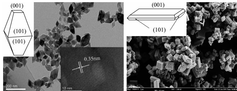
N-CDs doped octahedral bipyramids  $\text{TiO}_2$  with high exposed (101) reactive facets and N-CDs doped nanosheets  $\text{TiO}_2$  with high exposed (001) reactive facets have been successfully fabricated and their photodegradation performance were compared.
