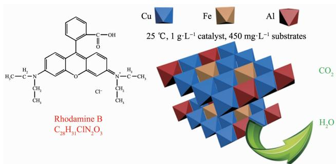
Layered  $\text{Cu}_y\text{Fe}_{6-y}\text{Al}_2\text{O}_x$  catalysts were prepared and applied in the Fenton degradation reaction of high concentrated rhodamine B under mild condition.
