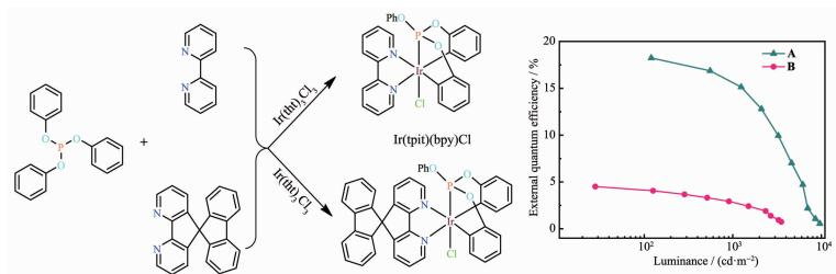
Based on the complex Ir(tpit)(sb)Cl containing spirofluorene group, the external quantum efficiency of OLED device is 4.5%. The external quantum efficiency of Ir(tpit)(bpy)Cl-based device is up to 18.2%.
