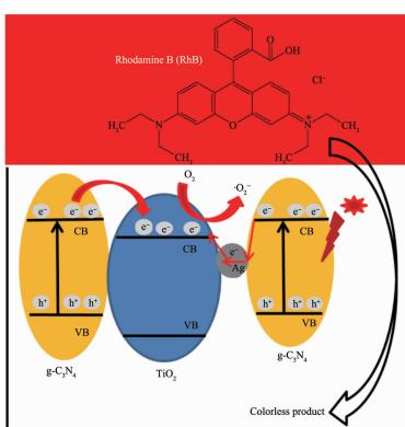
The  $\text{g-C}_3\text{N}_4/\text{Ag}/\text{TiO}_2$  composite photocatalyst with enhanced visible light activity for RhB degradation was facilely fabricated via a mechanical agitation procedure. The research shows  $\cdot\text{O}_2^-$  and  $\text{h}^+$  are the major reactive species, and the enhanced photocatalytic activity mainly contributed to the formation of heterojunction and the good conductivity of Ag.
